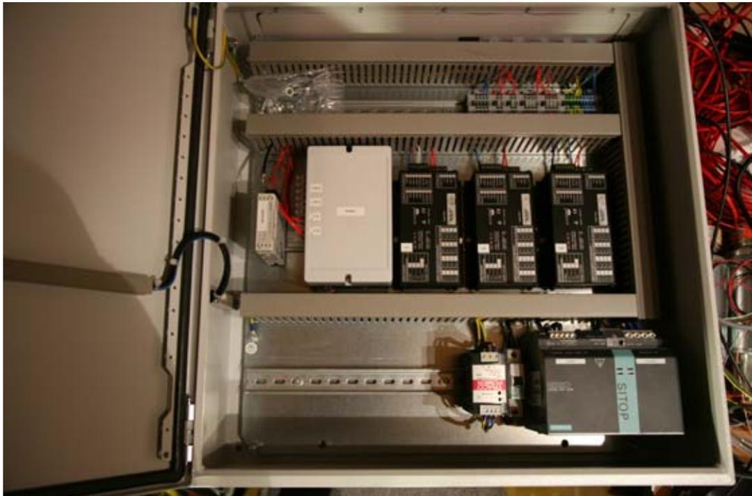
Electronics used to control the AltAz telescopes mounted in professional wall mounted enclosure
