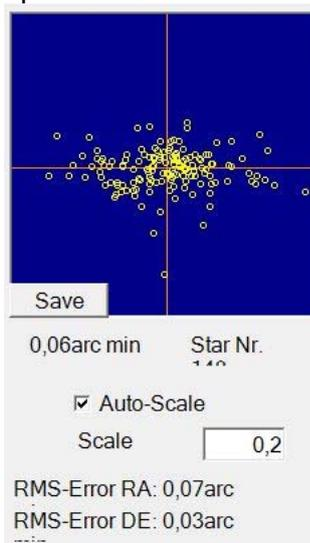
**Pointing accuracy: better than 5" RMS for each axis after pointing model correction (20degree > elevation < 75degree)**
