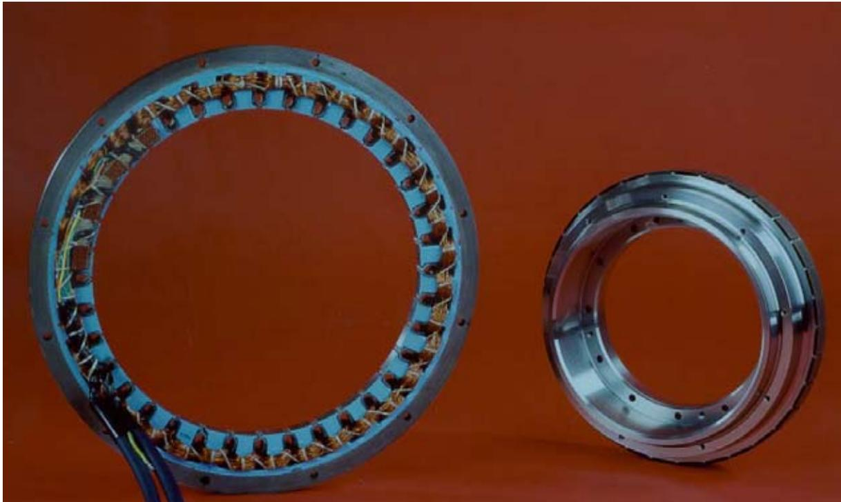
Our Torque motors are made in Germany by a company that makes special windings for these low speed applications that have a maximum Torque/Ampere factor. The motors used have a permanent Torque of 200NM (Peak 400NM) that can be reached with 48V and less than 20A. We wanted to avoid having 200V applied to the telescope (unsafe in humid environments).
