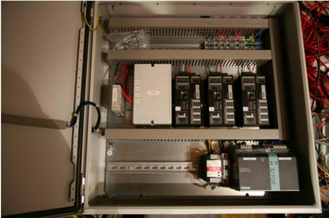
There is a wall mounted enclosure delivered with the telescope that should be mounted within 10m from the telescope and contains the power supply, servo amplifiers and some additional micro controllers. The enclosure is made by professional electronic engineers and is according to all common standards.
