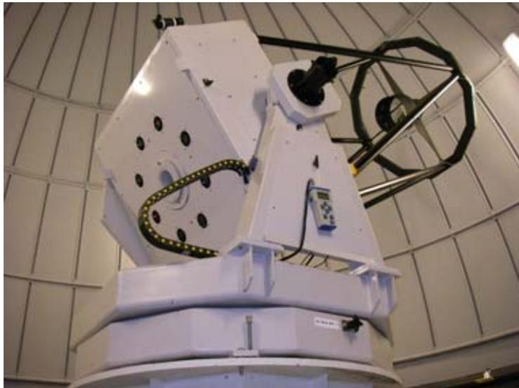
**Design 1 with conventional servo drive and dual loop encoder control), Example Stockholm Alba Nova University 1m:**
